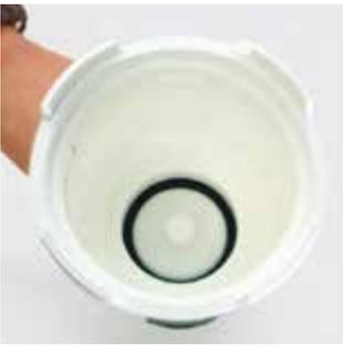
Reassemble your filter starting with the internal coalescer making sure you get a snug fit in the aluminum base. See **Figure 4**. Insert a new activated carbon filter, make sure you remove it from the shrink wrap and align the sight window with the adsorption indicator. See **Figure 5**. Finally, twist your weather cap back into place. See **Figure 6**.
