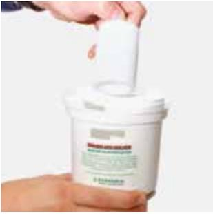
Remove the internal coalescer using the pull tab from the aluminum base. See **Figure 3**. Visually inspect the base for any standing liquids. If liquid has collected in the base drain the contents following the instructions provided on the green lower filter housing label.
