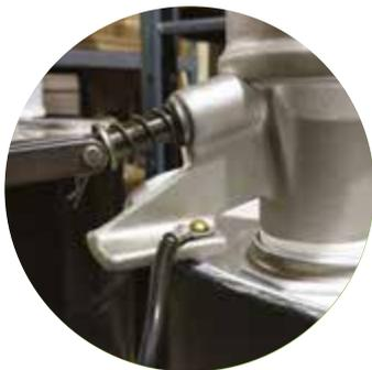
**4** Thread the aluminum filter base with the attached activated carbon filter into the 3/4” bung of the liquid collection drum - your system setup is now complete.
